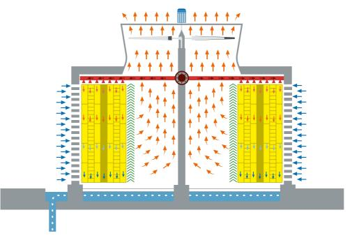
The Kelvion crossflow cooling tower operates quietly and economically and has a high cooling capacity. The modular system can be easily adjusted to suit cooling requirements and the space available. The cooling towers provide an optimal performance and problem-free operation. The considerable savings in water usage (95%+), and the exceptionally low noise level make the economical crossflow cooling towers the best choice for both people and the environment.
